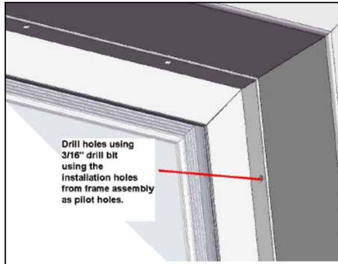
6. Secure using #8 x 1-1/4" screws provided.
