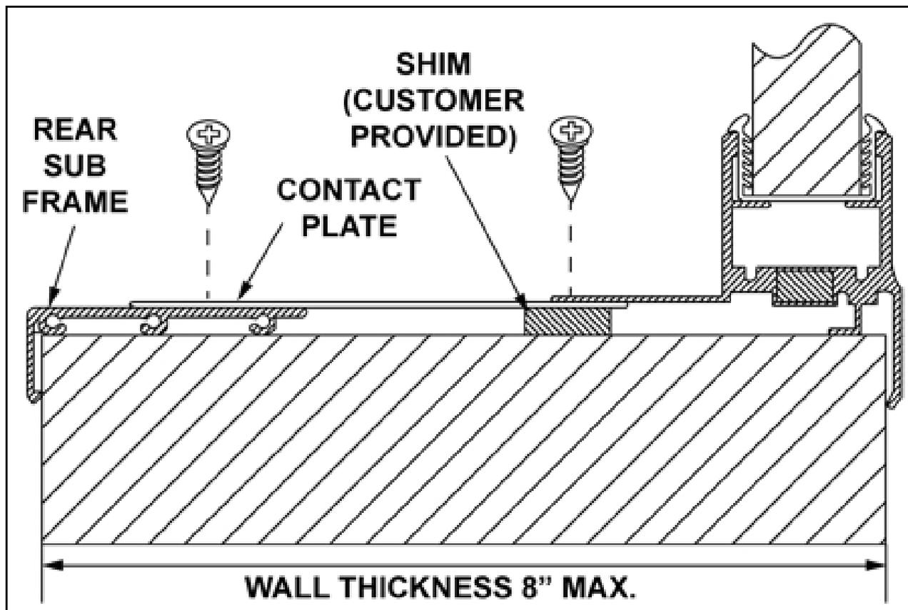
**NOTE:** An additional contact plate must be requested for specific wall widths of over 6-1/4"
