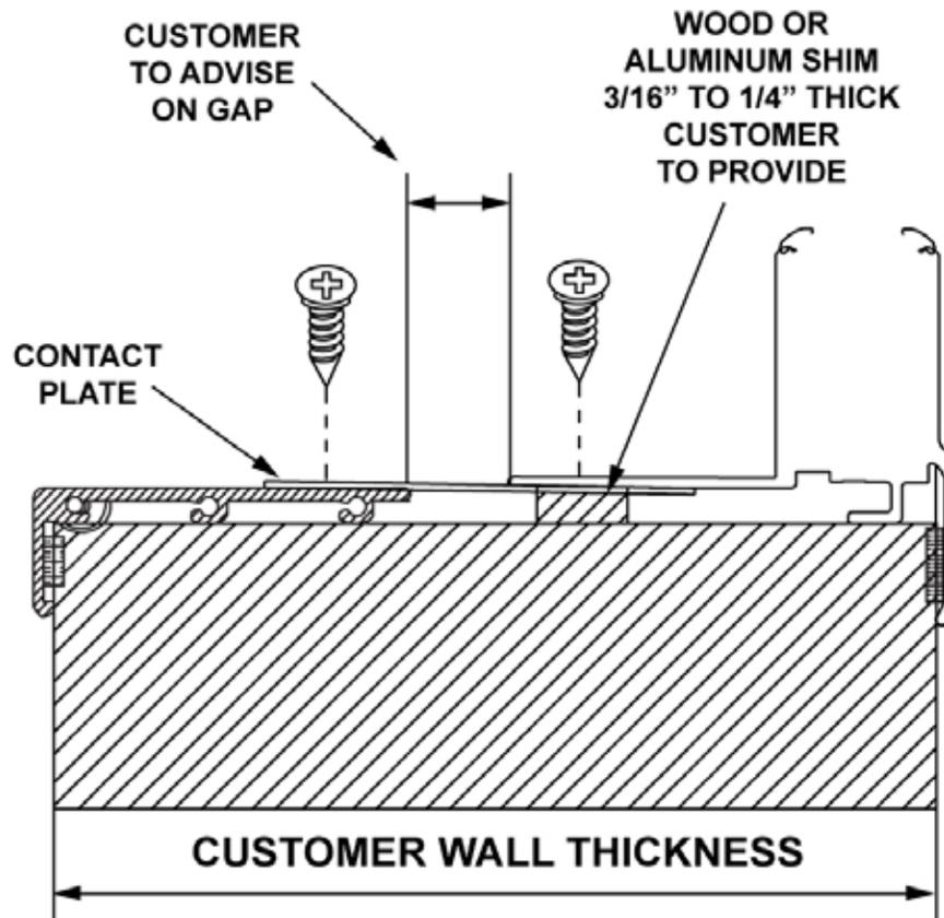
5. Drill holes using a 3/16" drill bit using only the installation holes from the frame assembly as pilot holes.
