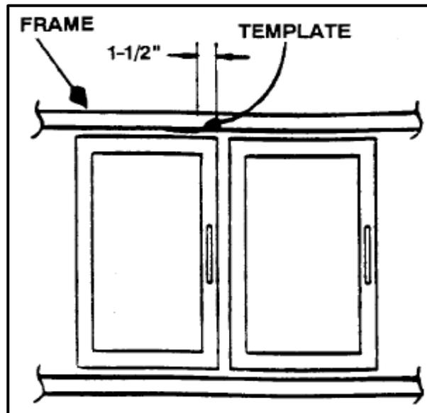
2. Place the template provided on the frame with the right edge of the template on the mark created in Step 1.
