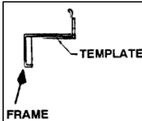
3. Mark the frame through the five holes on the template with a pencil. Remove the template and center punch the marks on the frame.
