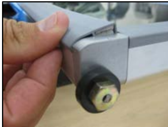
Insert Plastic Cover Outer Edge
