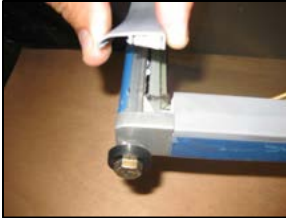
Disengage Plastic Rail
