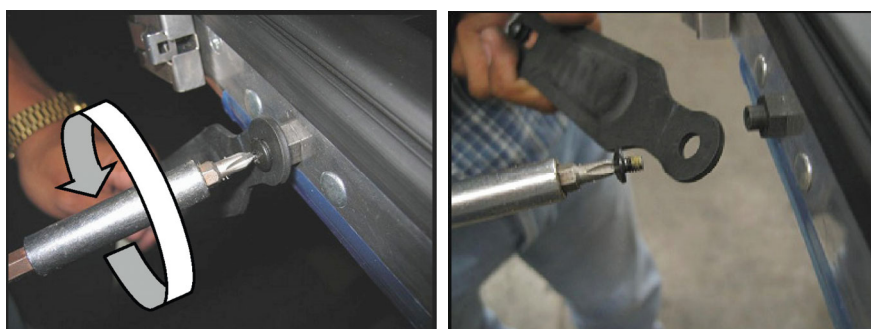
Figure 13.1 Removing hold-open assembly from door.
