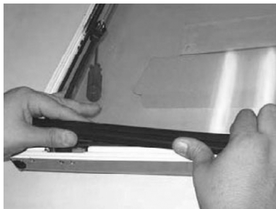
Figure J.3 – Separating Plastic Cover from the door rail
