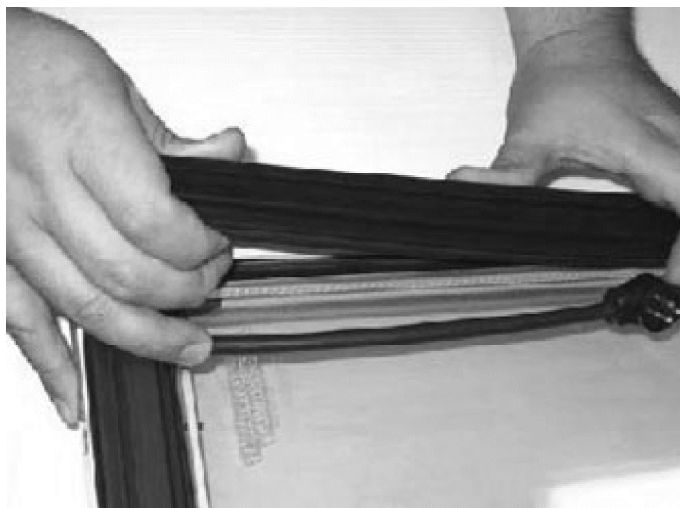
Figure J.4 – Installing replacement Plastic Cover
