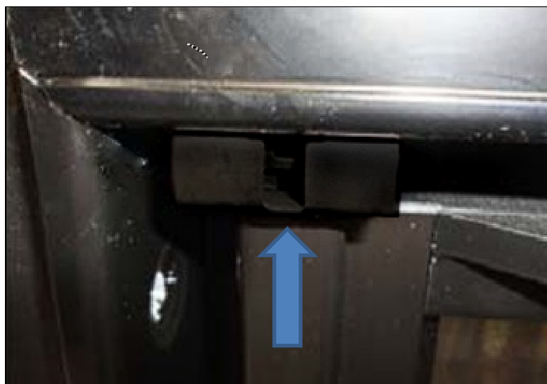
Figure 4.2: Engage Hinge Pin to Frame
