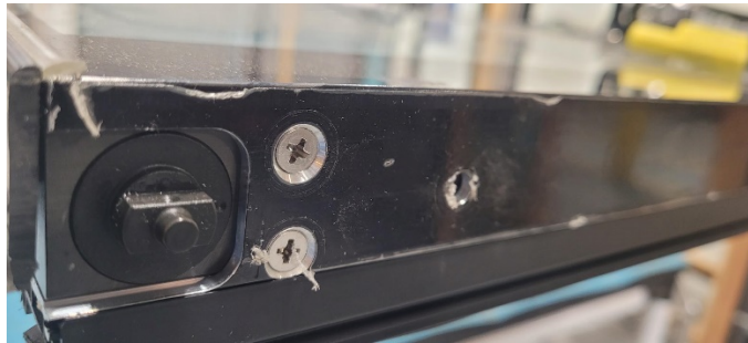
Figure 2.1 Hydraulic hinge tab at “Zero-degree” position
