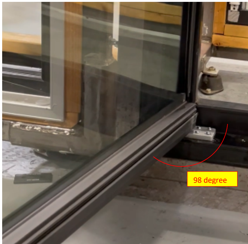
Figure 3.1 Seating door into hydraulic hinge adapter plate.
