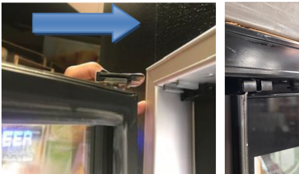
Figure 4.1 Insert Door Hinge Pin to Frame Socket
