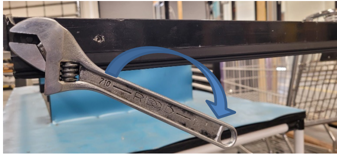
Figure 2.2 Rotating clockwise using at least a 10" crescent wrench.
