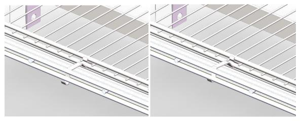
4. Attach price tag molding to the LED bracket, as shown in the following illustration.
