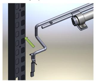
2. Turn thumb knobs clockwise to lock bracket in place at both ends and attach shelf to post right above LED/bracket assembly, as shown.
