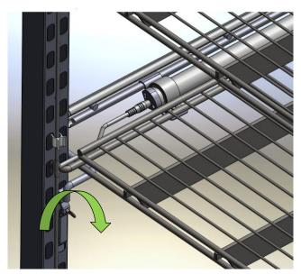
3. Install hooks approximately at the midpoint of the shelf, starting on the shelf then snap the J-hook to the bottom rod of the bracket, creating a bridge between the shelf and LED bracket, as shown in the following illustration.
