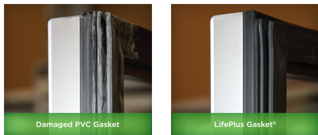
Figure 1: Comparison of competitor PVC gasket versus LifePlus Gasket, showing superior performance of LifePlus Gasket after 80,000 cycles.
