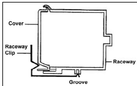
1. Insert flat-head screwdriver under top edge of clip and lift to remove.
