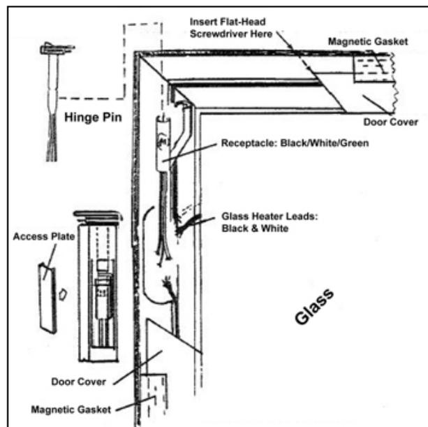
2. Unplug molded hinge pin plug at heater access hole and remove hinge pin out through top of door. Remove heater wire from perimeter of door.
