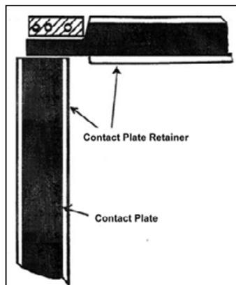
2. Insert new plastic retainer with correct plates on horizontal sections first, then vertical sections. Insert outer edge of plastic into groove in frame. Snap inner edge into grooves of inner edge of frame.
