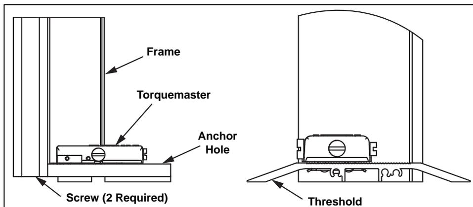
*Pass-Thru Cross-Section (with/without Threshold)*
