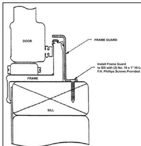
2. Install protector to sill with three (3) No. 10 x 1" Hi-Lo Phillips screws provided into pre-drilled holes.
