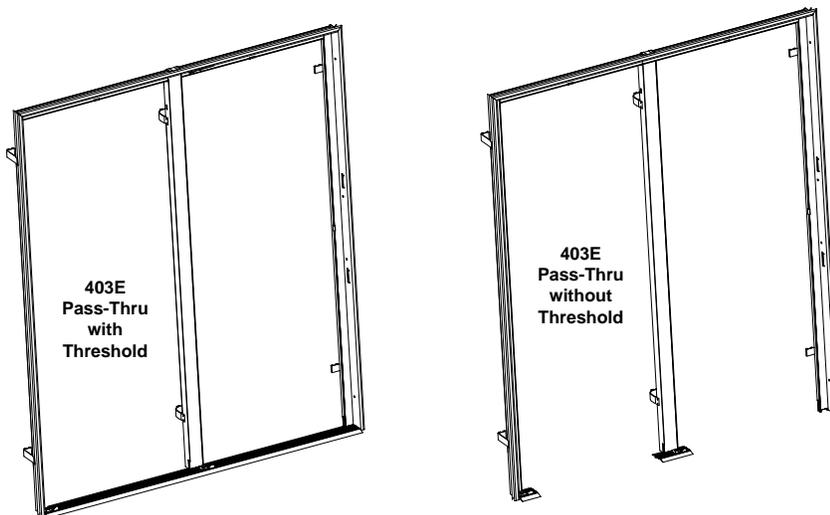
2. When no threshold is desired, drill and lag on pre-drilled mounting holes only.
