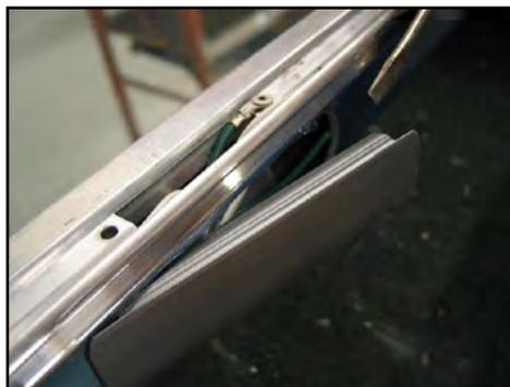
2. Insert flat-head screwdriver under edge of cover and gently lift up.
