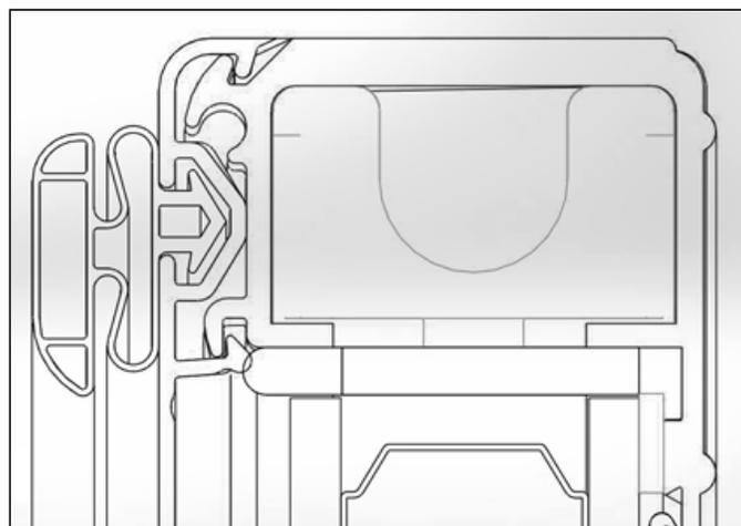
2. To replace, start at bottom of door. Insert gasket into groove in both sides of door and slide gasket up to top of door. Tuck in all four corners with flat-head screwdriver.
