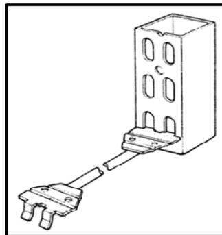
2. Insert the forked end of stabilizer bar into the elongated holes in post.
