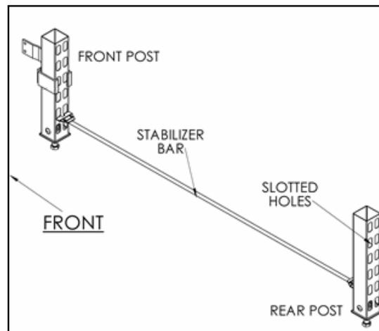
3. Install the post stabilizers on top and bottom of all posts, front to rear, before installing shelves.
