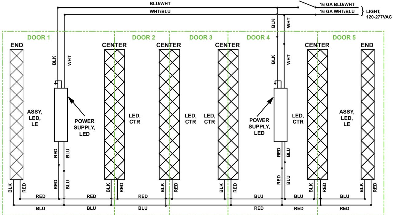
8. Model 401 Optimax Pro 24V Wiring Diagram (6-Door: 48" & 54" Low Power)
