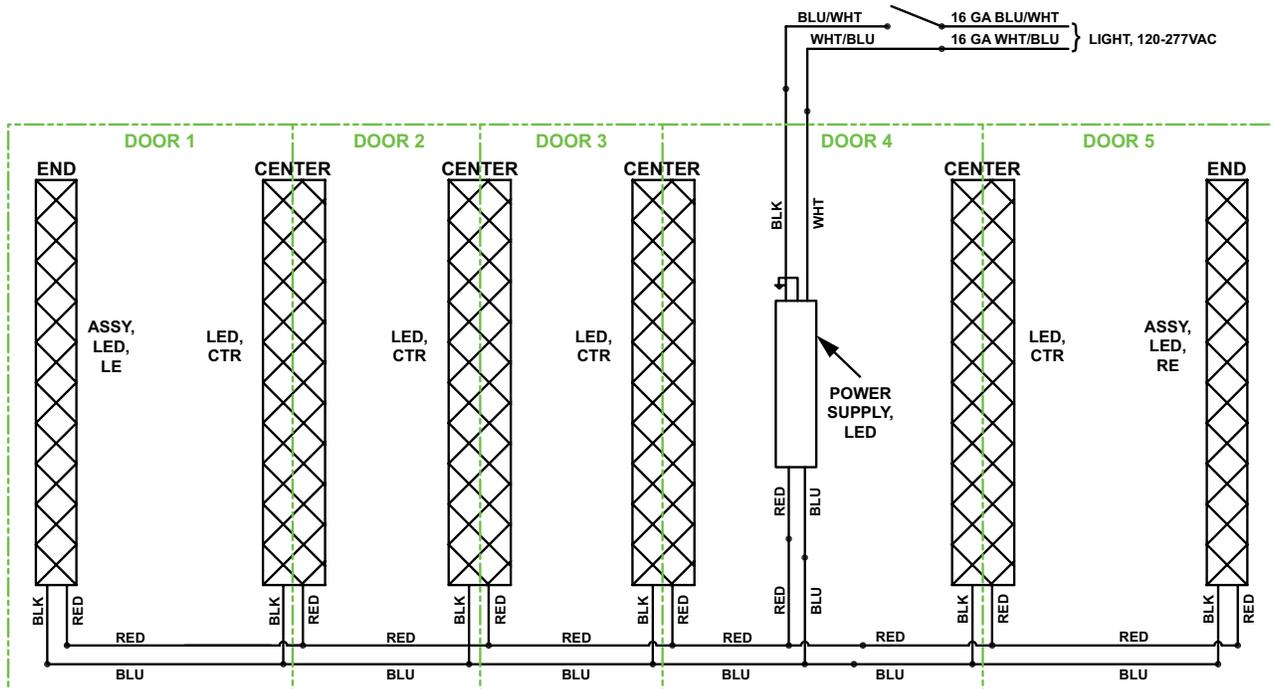
7. Model 401 Optimax Pro 24V Wiring Diagram (5-Door: 54", 60" & 72" High Power)
