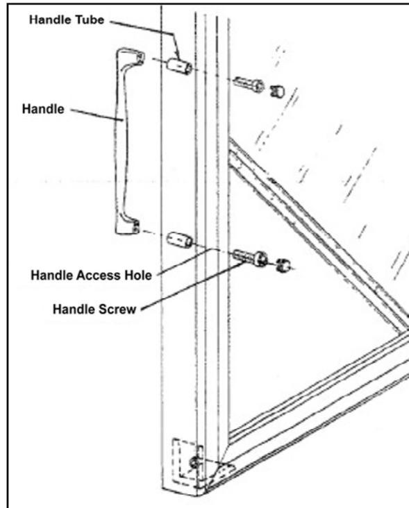
2. Insert 5/32" Allen wrench into access holes and remove screws.
