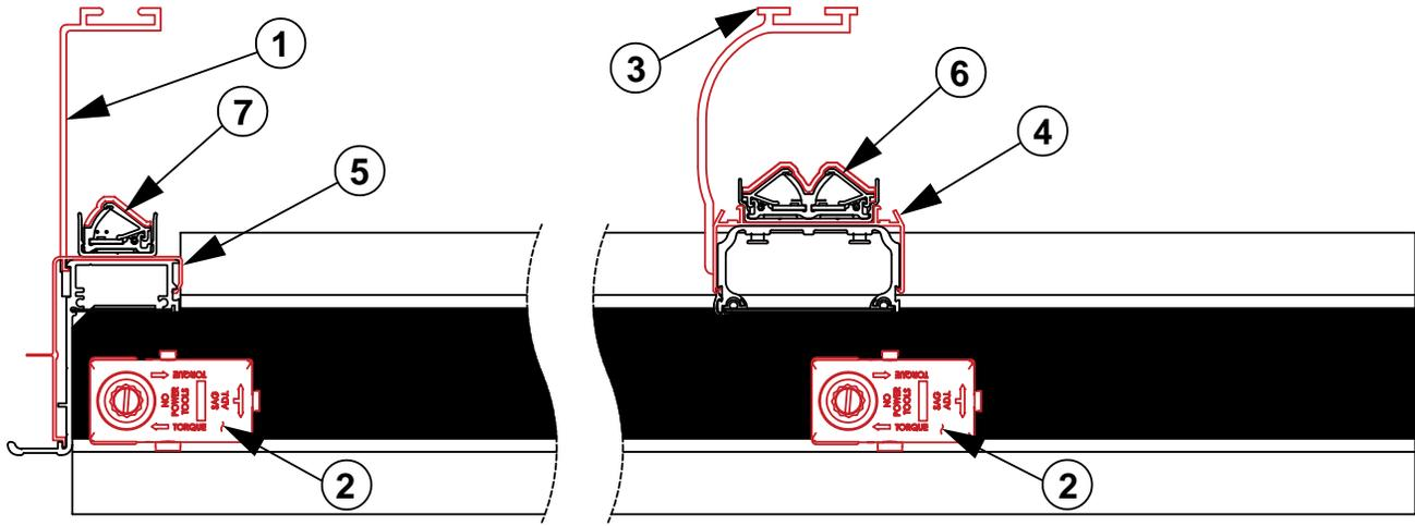
**SECTION: D** Pass-Thru with Threshold
