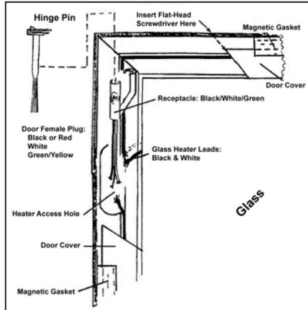
2. Unsnap female receptacle from hinge pin and remove hinge pin out through top of door. Then pull receptacle out of access hole and cut lead wires to replace.
