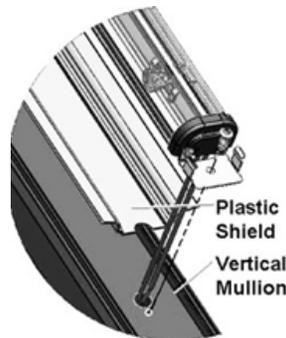
8. Use a power drill and (3/8") 0.375" dia. drill bit, drill (1) hole.
