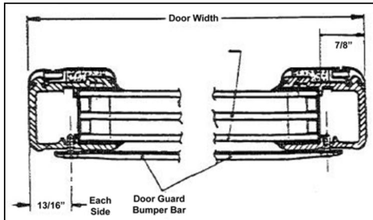
3. Anthony provides pre-drilled screw holes in bar. Customer must drill a #30 or 1/8" hole in door rail 13/16" in from each side of door rail.
