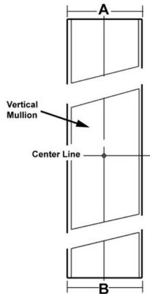
2. Mark a vertical line from the top of the Mullion to the bottom of the Mullion through the lines measured in step 1.
