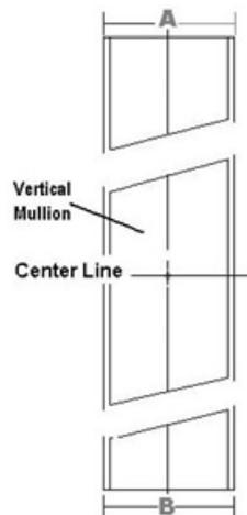
2. Mark a vertical line from the top of the Mullion to the bottom of the Mullion through the lines measured in step 1.
