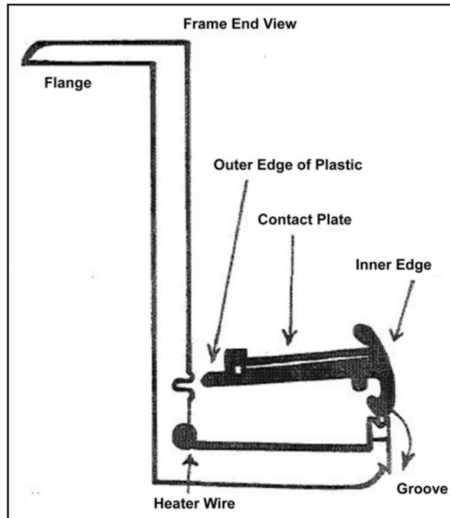
3. Work on 6" sections at a time. If you try to work on a larger area, plastic will not stay in place. Trim contact plates if necessary
