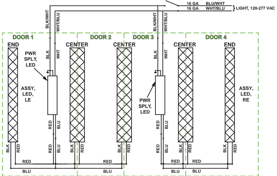
6. Model 401 Optimax Pro 24V Wiring Diagram (5-Door: 48" High Power & All Low Power)
