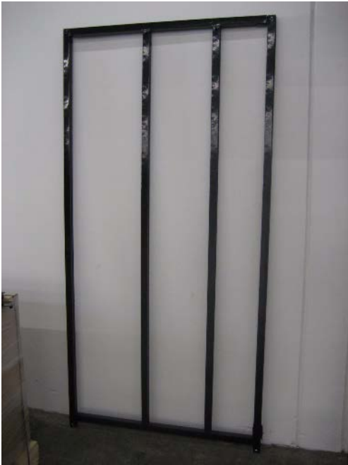
Figure 5 Upright welded assembly
