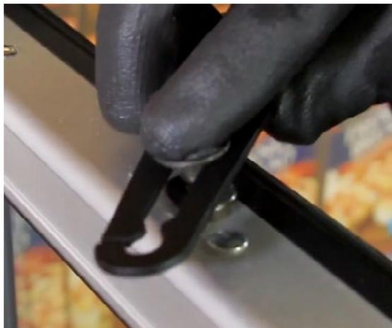
4. Insert the washer and the hold-open bolt into the frame mounting hole and tighten the bolt, use a 7/16" open-ended hand wrench.
