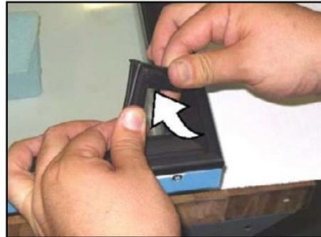
2. Carefully pull the gasket out of the groove in the plastic rail covers.
