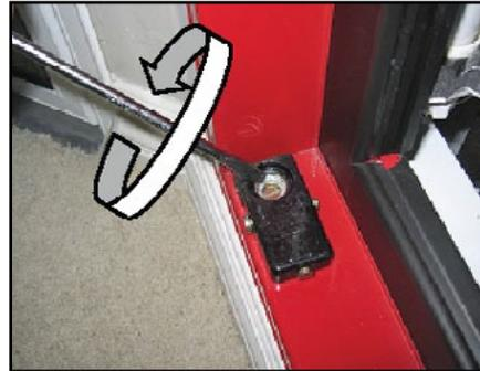
2. Remove the Torquemaster from the frame mount.
