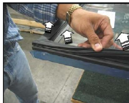
**NOTE:** The gasket is composed of soft materials with welded miter joints. Use extra care when manually extracting the gasket from the rail grooves to prevent damaging it as well as the plastic rail.
