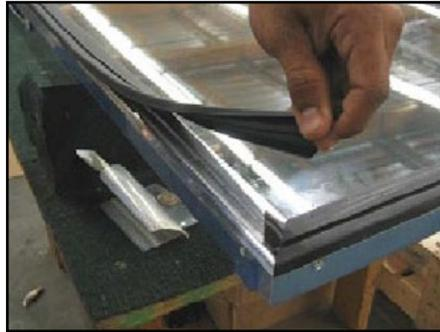
4. Pull the plastic cover up and out of door rail grooves until the entire plastic cover is removed from the door rail.
