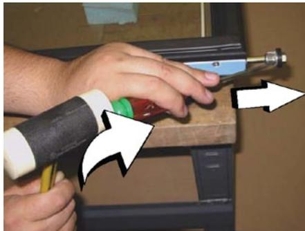
**NOTE: Use caution when striking any tool with another tool. DO NOT use excess force when striking the screwdriver and potentially damaging the door.**
