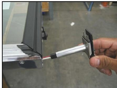
4. Upon replacing the hinge pin, insert all three wires into the hinge pin hole in the door rail.
