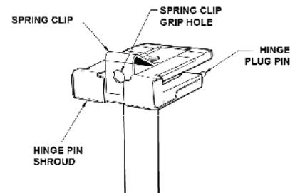
**Figure 15 Hinge Pin Assembly**
