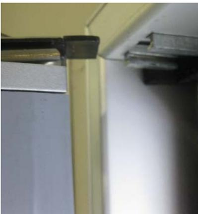
**Figure 13 Withdraw Away From Hinge Gib**
