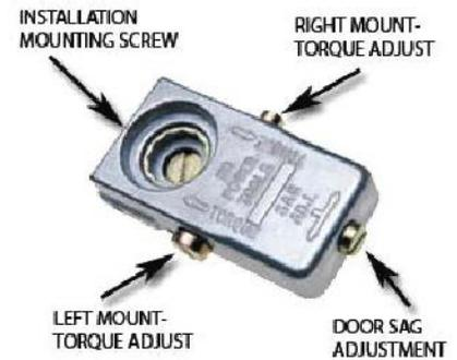
Figure 16 TorqueMaster Assembly
