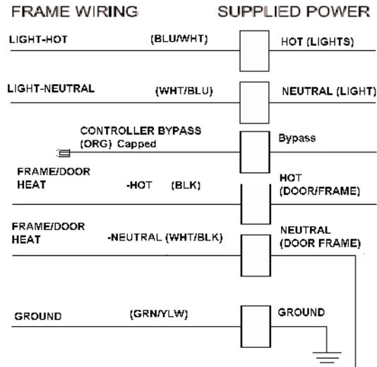
**Figure 5 Wiring W/ Energy Controller**
